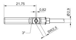
$1^*$  = switching point  $2^*$  = locking screw  $3^*$  = LED window, transparent
