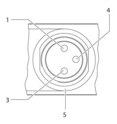
PIN assignment: 1) PIN not assigned 3) 0 V 4) 24 V 5) LED Cable color 1)
