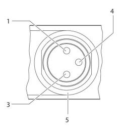
PIN assignment: 1) PIN not assigned 3) 0 V 4) 24 V 5) LED Cable color 1) Brown 3) Blue 4) Black
