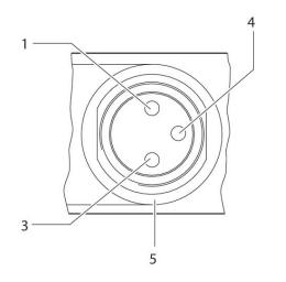
PIN assignment: 1) PIN not assigned 3) 0 V 4) 24 V 5) LED Cable color 1) Brown 3) Blue 4) Black Note: Bi-polar protective circuit to prevent overvoltage
