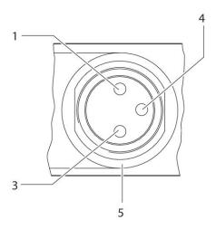
PIN assignment: 1) PIN not assigned 3) 0 V 4) 24 V 5) LED Cable color 1) Brown 3) Blue 4) Black
