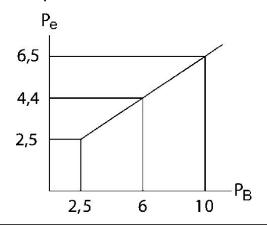
Pe = external control pressure, min.
