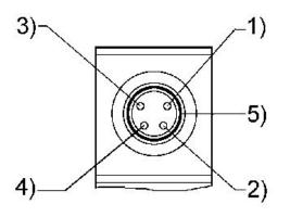
PIN assignment: 1) PIN not assigned 2) PIN not assigned 3) 0 V 4) 24 V 5) LED Cable colors 1) Brown 2) White 3) Blue 4) Black
