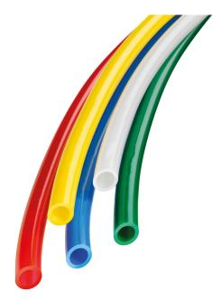
Industrial suitable for dynamic laying 10 mm 1.25 mm 45 mm Blue -30 °C 80 °C 10 bar 50 m 0.042 kg Polyester polyurethane R412009991
