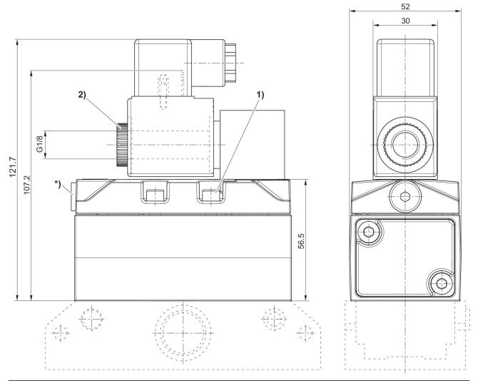
Tightening torque for mounting screws: 2.2 ± 0.2 Nm
