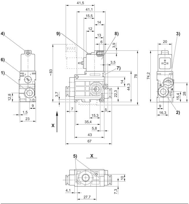
1) Port 1 2) Port 2 3) Port 3, exhaust air must not be throttled 4) Core Ø for M5 5) Pocket hole 6 mm deep for 3.5 self-tapping screw 6) Manual override 7) Mounting space for name plate 8) Coil can be rotated at 180° intervals 9) LED
