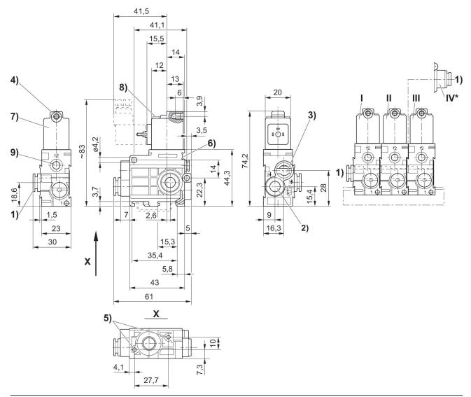
1) Port 1 2) Port 2 3) Port 3, exhaust air must not be throttled 4) Core Ø for M5 5) Pocket hole 6 mm deep for 3.5 self-tapping screw 6) Mounting space for name plate 7) Coil can be rotated at 180° intervals 8) LED 9) Port 12 \* Air connection module (item IV) mounted onto stacking valve (item II) permits additional air supply from right hand side. End valve (item III) not required. I = Inlet valve, II = Stacking valve, III = End valve
