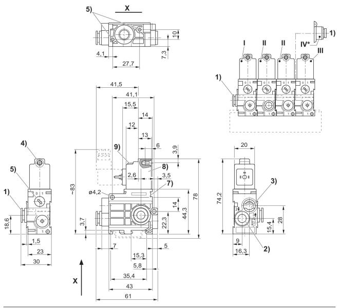
1) Port 1 2) Port 2 3) Port 3, exhaust air must not be throttled 4) Core Ø for M5 5) Manual override 6) Pocket hole 6 mm deep for 3.5 self-tapping screw 7) Mounting space for name plate 8) Coil can be rotated at 180° intervals 9) LED \* Air conn. module (item IV) mounted onto stacking valve (item II) permits additional air supply from right hand side. End valve (item III) not required.
