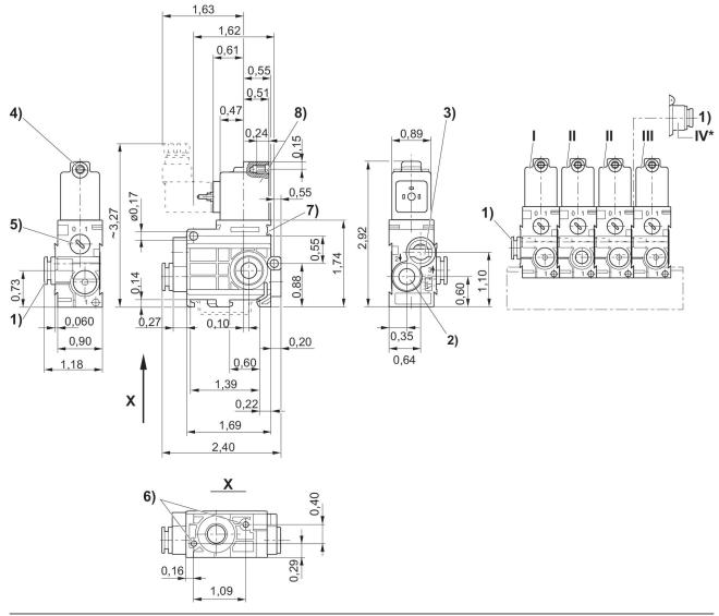
1) Port 1 2) Port 2 3) Port 3, exhaust air must not be throttled 4) Core Ø for M5 5) Manual override 6) Pocket hole 6 mm deep for 3.5 self-tapping screw 7) Mounting space for name plate 8) Coil can be rotated at 180° intervals \* Air conn. module (item IV) mounted onto stacking valve (item II) permits additional air supply from right hand side. End valve (item III) not required.
