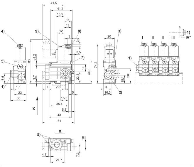
1) Port 1 2) Port 2 3) Port 3, exhaust air must not be throttled 4) Core Ø for M5 5) Manual override 6) Pocket hole 6 mm deep for 3.5 self-tapping screw 7) Mounting space for name plate 8) Coil can be rotated at 180° intervals 9) LED \* Air conn. module (item IV) mounted onto stacking valve (item II) permits additional air supply from right hand side. End valve (item III) not required.
