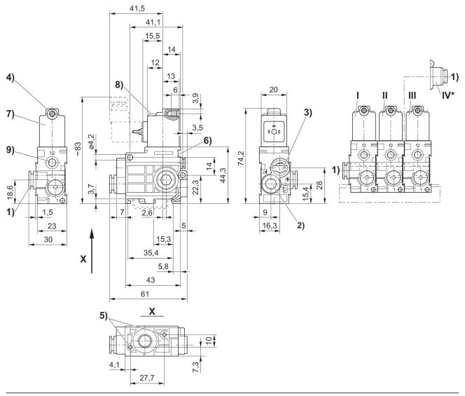
1) Port 1 2) Port 2 3) Port 3, exhaust air must not be throttled 4) Core Ø for M5 5) Pocket hole 6 mm deep for 3.5 self-tapping screw 6) Mounting space for name plate 7) Coil can be rotated at 180° intervals 8) LED 9) Port 12 \* Air connection module (item IV) mounted onto stacking valve (item II) permits additional air supply from right hand side. End valve (item III) not required.
