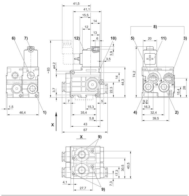
1) port 1 2) port 2 3) port 3 4) port 4 5) port 5 6) manual override 7) core Ø for M 5 8) exhaust air must not be throttled 9) pocket hole 6 mm deep for 3.5 self-tapping screw 10) mounting space for name plate 11) coil can be rotated at 180° intervals
