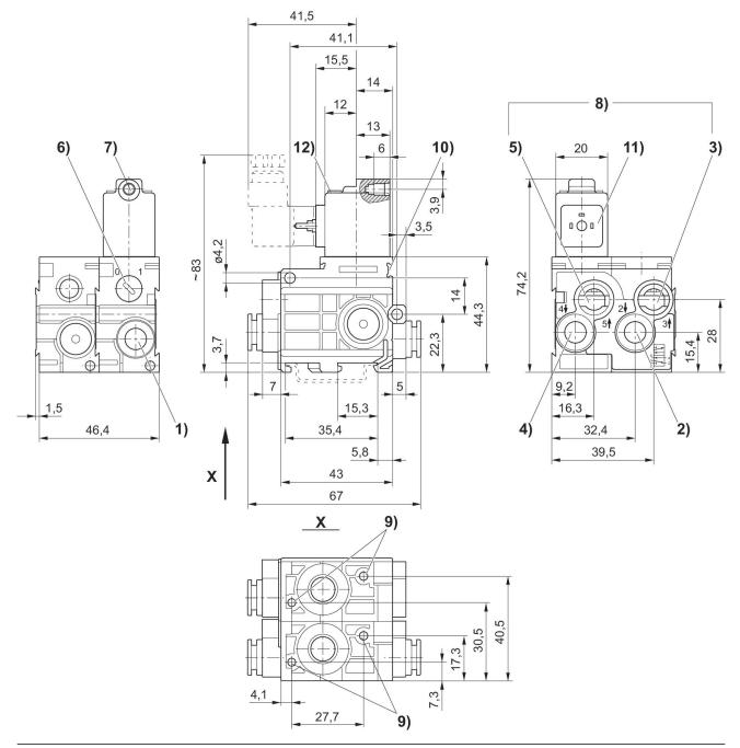
1) port 1 2) port 2 3) port 3 4) port 4 5) port 5 6) manual override 7) core Ø for M 5 8) exhaust air must not be throttled 9) pocket hole 6 mm deep for 3.5 selftapping screw 10) mounting space for name plate 11) coil can be rotated at 180° intervals
