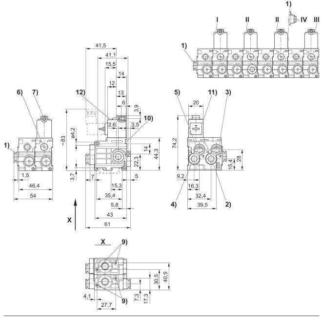
1) Port 1 2) Port 2 3) Port 3 4) Port 4 5) Port 5 6) Manual override 7) Core Ø for M5 8) Exhaust air must not be throttled 9) Pocket hole 6 mm deep for 3.5 self-tapping screw 10) mounting space for name plate 11) Coil can be rotated at 180° intervals 12) LED \* Air connection module (item IV) mounted onto stacking valve (item II) permits additional air supply from right hand side. End valve (item III) not required.
