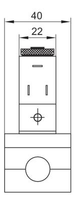
The pilot valves can be loosened and turned through 180°.
