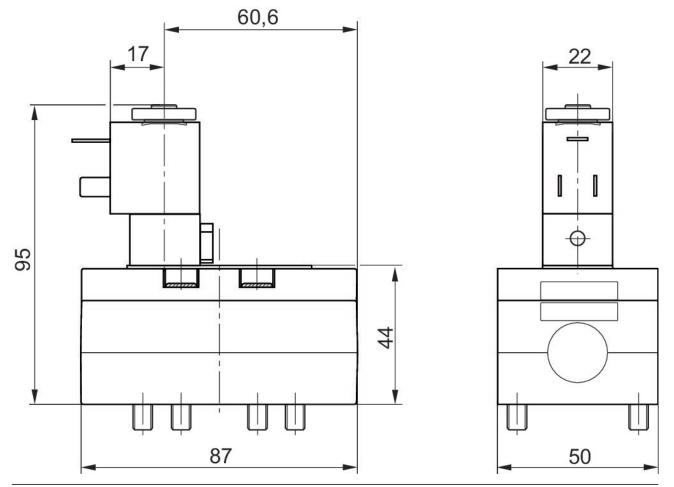
The pilot valves can be loosened and turned through 180°.
