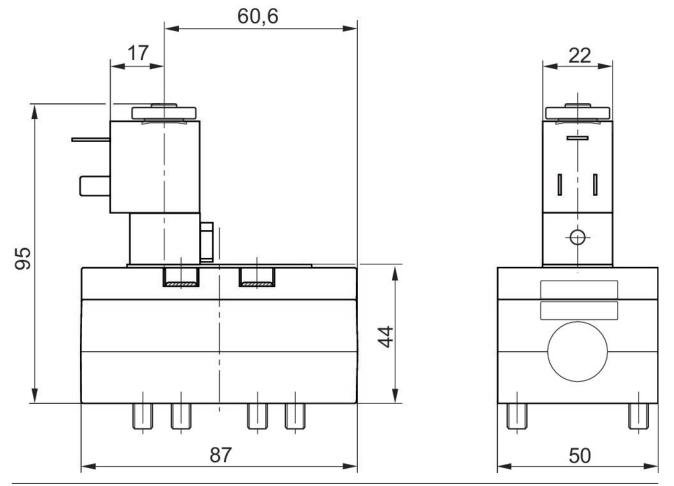
The pilot valves can be loosened and turned through 180°.
