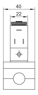
The pilot valves can be loosened and turned through 180°.
