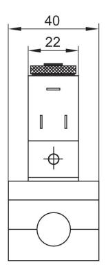
The pilot valves can be loosened and turned through 180°.
