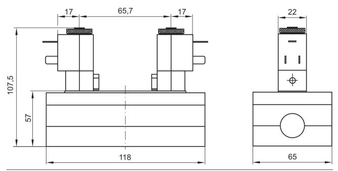
The pilot valves can be loosened and turned through 180°.
