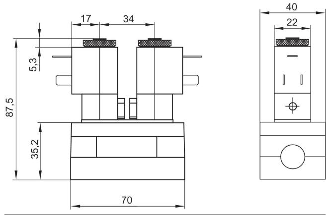
The pilot valves can be loosened and turned through 180°.
