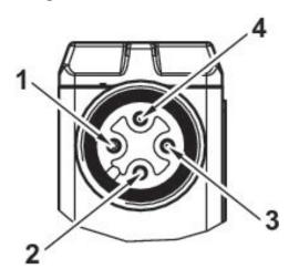
1) not assigned 2) Coil 12 3) 0 V DC 4) Coil 14
