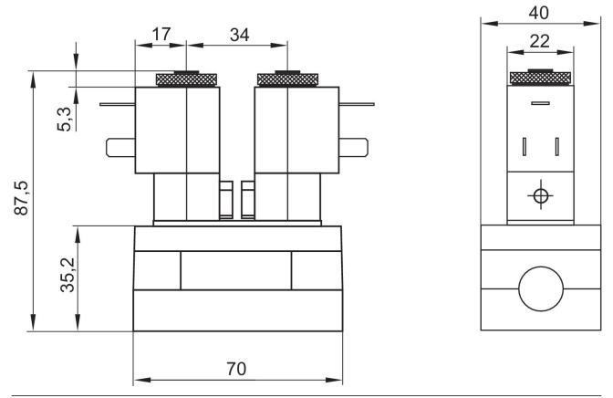
The pilot valves can be loosened and turned through 180°.
