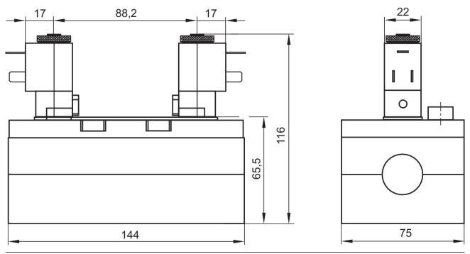
The pilot valves can be loosened and turned through 180°.
