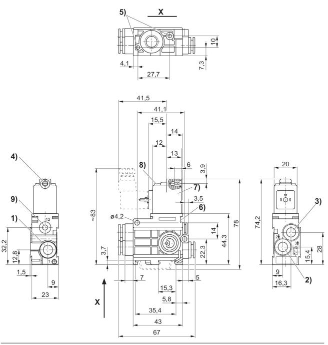
1) port 1 2) port 2 3) port 3 4) core Ø for M 5 5) pocket hole 6 mm deep for 3.5 self-tapping screw 6) mounting space for name plate 7) coil can be rotated at 180° intervals 8) LED 9) port 12
