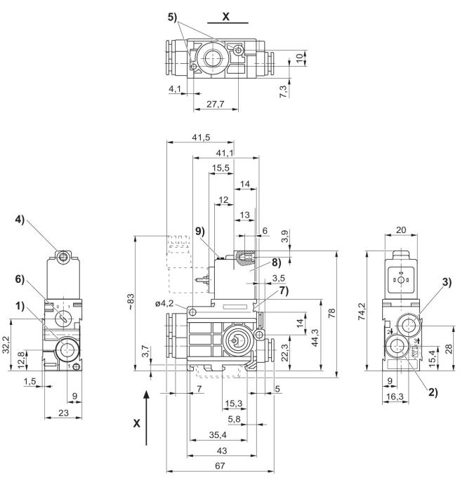
1) port 1 2) port 2 3) port 3 4) core Ø for M 5 5) pocket hole 6 mm deep for 3.5 self-tapping screw 6) manual override 7) Pilot valve 8) coil can be rotated at 180° intervals
