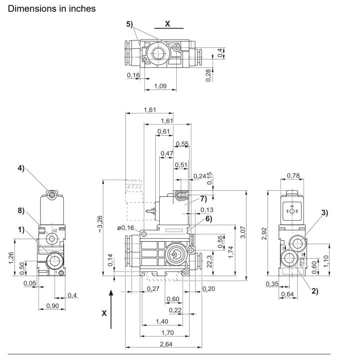
1) port 1 2) port 2 3) port 3 4) Ø for M 5 5) pocket hole 6 mm deep for 3.5 self-tapping screw 6) mounting space for name plate 7) coil can be rotated at 180° intervals 8) port 12
