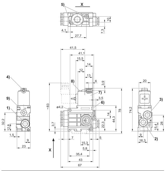
1) port 1 2) port 2 3) port 3 4) Ø for M 5 5) pocket hole 6 mm deep for 3.5 self-tapping screw 6) mounting space for name plate 7) coil can be rotated at 180° intervals 8) LED 9) port 12
