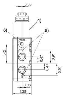
Manual actuation: (1) with detent - push and turn into position 1 (2) without detent - remove segment I - push only Actuation with tool: (3) with detent - remove segments up to II - push with tool and turn into position 1
