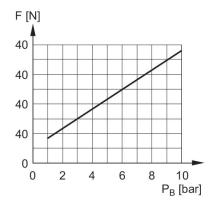
F = actuating force P<sub>B</sub> = Working pressure
