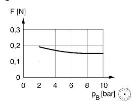
F = actuating force at the rear end of the spring-loaded rod  $P_B$  = Working pressure
