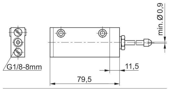
Mounting via 2 through-holes in housing
