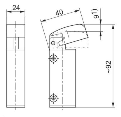
1) Actuating stroke Mounting via 2 through-holes in housing
