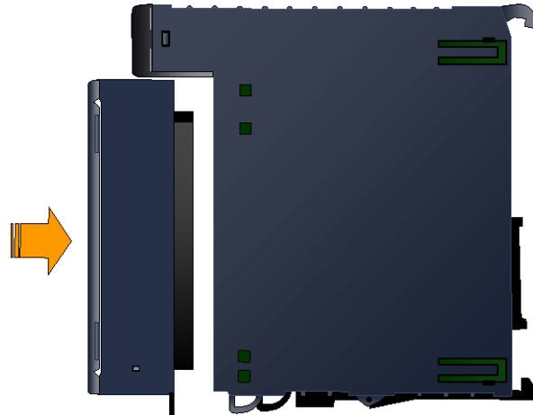
Figure 443: Installing a High-Density Terminal Block
