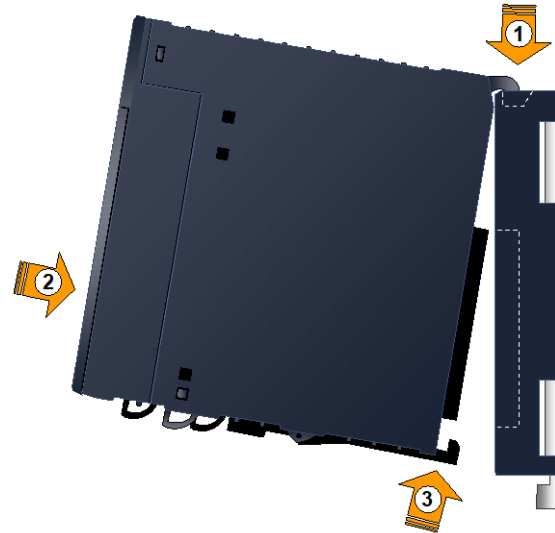
Figure 23: Installing Module in Backplane
