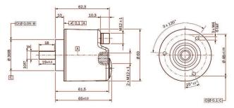
Diameter x f7 corresponds to the shaft diameter Solid shaft, face mount flange
