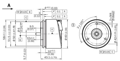
① Cable diameter = 5.6 mm + /-0.2 mm bend radius = 30 mm
