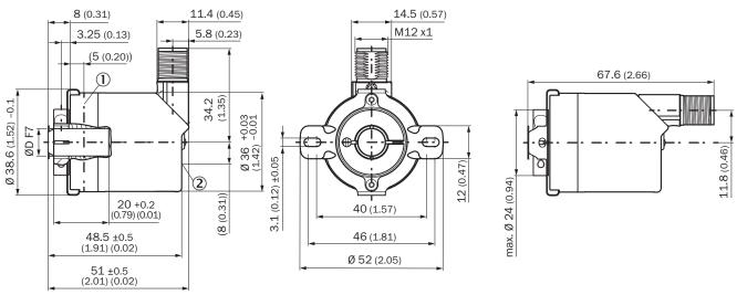
① Measuring point for operating temperature
