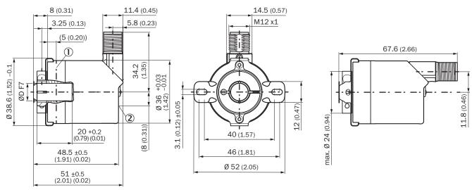
① Measuring point for operating temperature② Measuring point for vibrations
