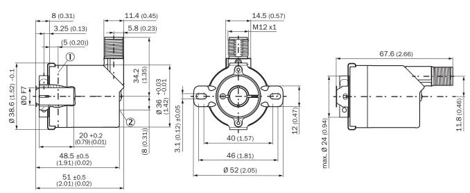
① Measuring point for operating temperature
