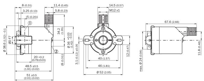
① Measuring point for operating temperature
