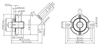
Non-tolerated dimensions according to DIN-ISO 2768-mk ① Measuring point for operating temperature ② Measuring point for vibrations
