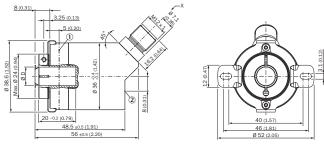
Non-tolerated dimensions according to DIN-ISO 2768-mk
