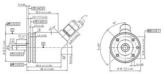
Non-tolerated dimensions according to DIN-ISO 2768-mk
