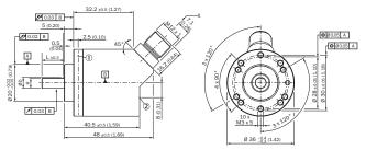
Non-tolerated dimensions according to DIN-ISO 2768-mk
