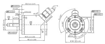
Non-tolerated dimensions according to DIN-ISO 2768-mk
