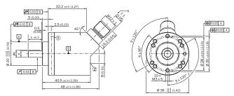
Non-tolerated dimensions according to DIN-ISO 2768-mk
