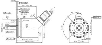
Non-tolerated dimensions according to DIN-ISO 2768-mk
